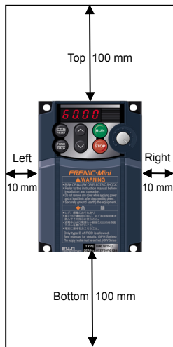
Figure 2.1 Mounting Direction and Required Clearances
