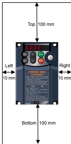
Figure 2.1 Mounting Direction and Required Clearances
