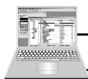
FRENIC loader Allows operation of the inverter connected on-line with the PC.
